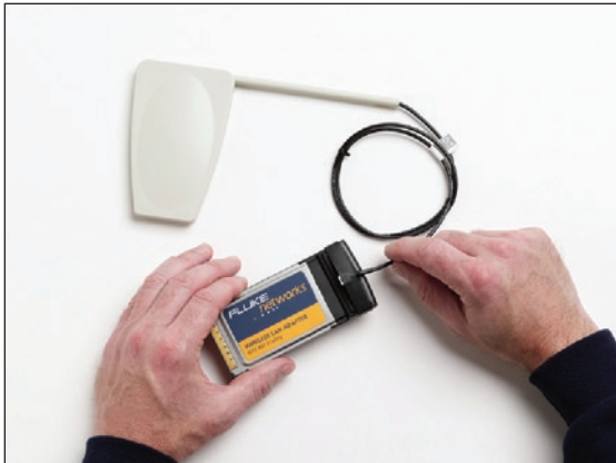
Figure 7 - Card with external unidirectional antenna
